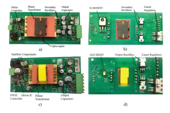
Aim of this project is to determine the viability of GaN HEMT for dc-dc converter applications for space, military and aircraft applications. There is a need to generate multiple low voltages for different electronics. This project intents to utilize GaN HEMT for this application. The project involves study, design, simulation and prototype development of dc-dc converter.
